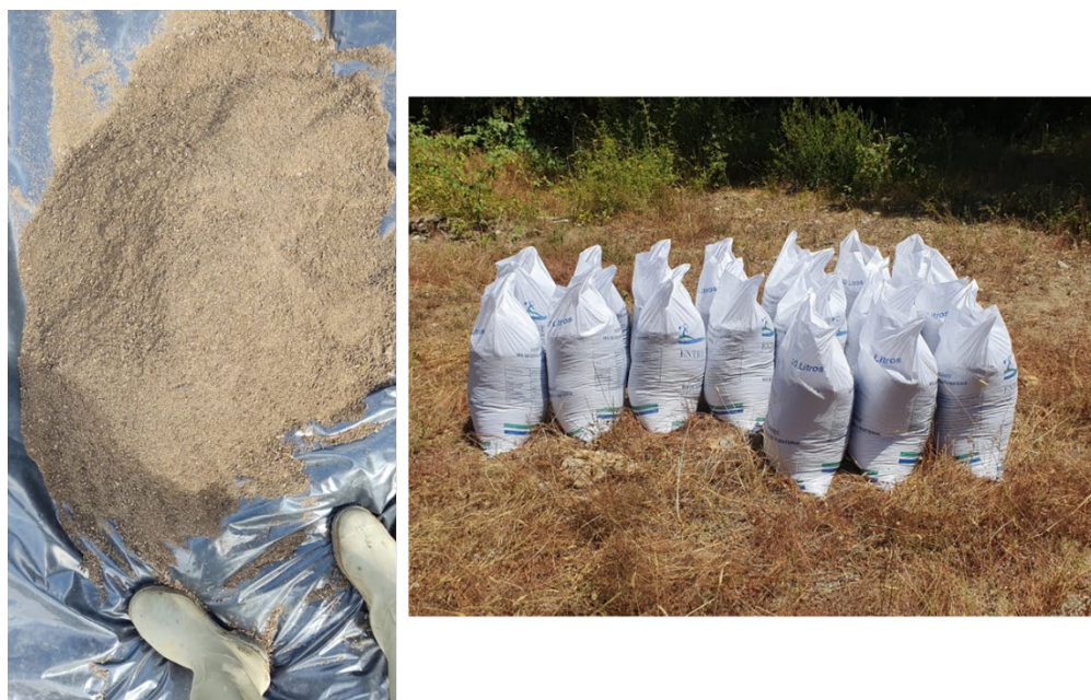
Figure 6: Dried sludge (left) and bagged for delivery (right). Images provided by Juan Villasante, Piscicola Entre Rios.
