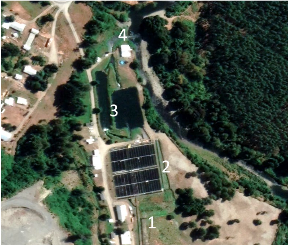
Figure 1: Aerial view of a freshwater raceway trout farm in Chile: 1) water supply channel from upstream water intake in the river; 2) raceways; 3) settling ponds; and 4) water return to river. Image reproduced from Google Earth.
