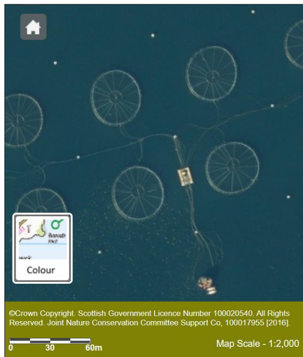
Figure 12: Closer view of the same Scottish salmon farm showing the feed barge at the bottom of the picture, the floating feed distribution pipes leading to each of the twelve net pens, and the surface components of the mooring
