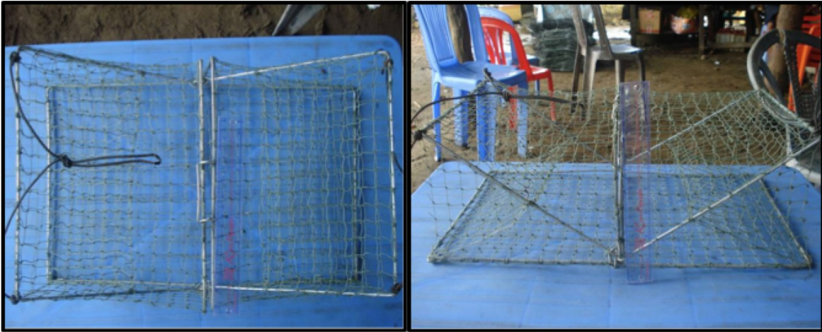
Figure 2: Normal crab trap used in the Vietnam blue swimming crab fishery. Photo from Thuy Nyugen.
