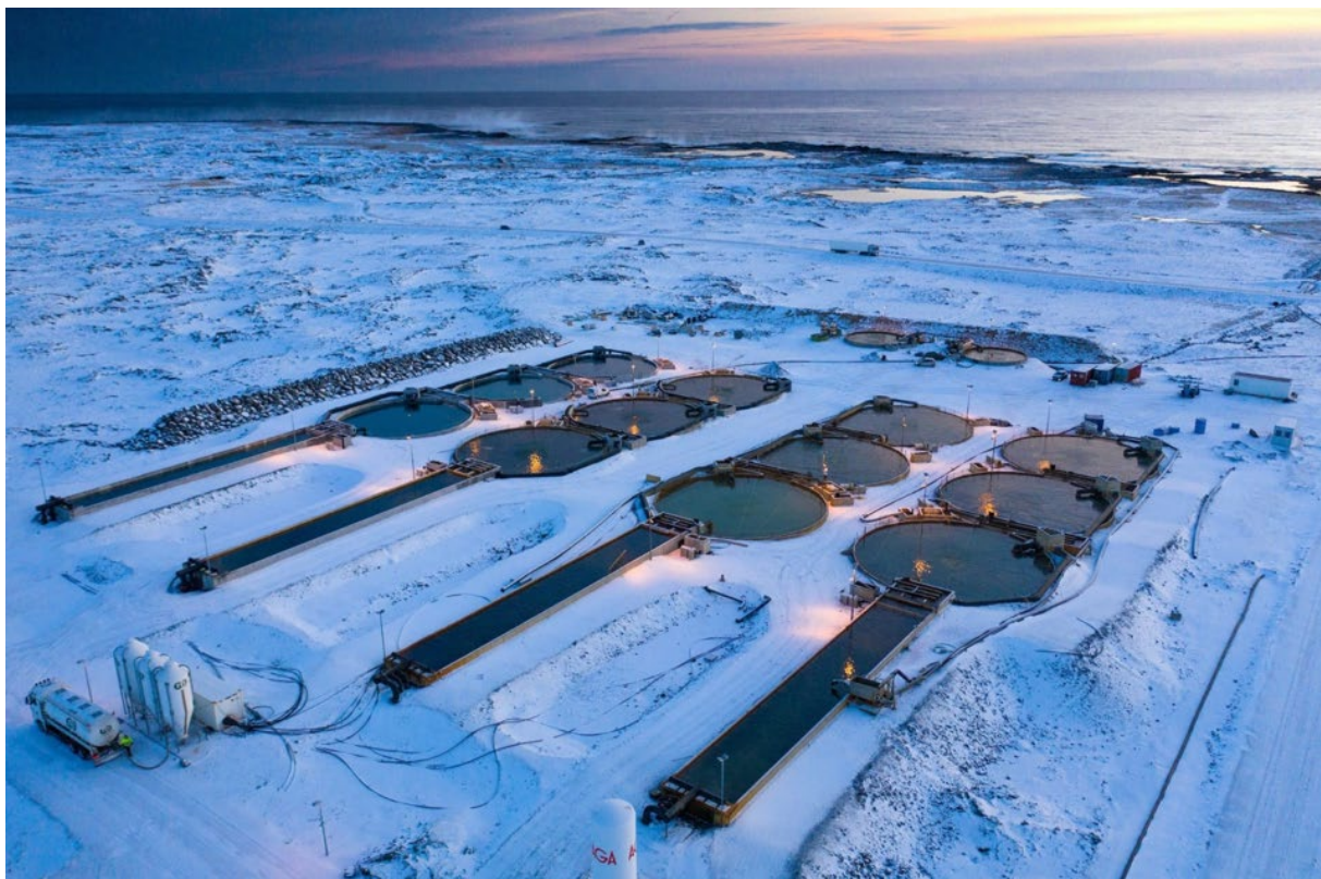
Figure 7: Aerial view of a land-based PRAS Arctic charr farm on Iceland's southwest coast near Grindavík. (Photo credit: Matorka.)
