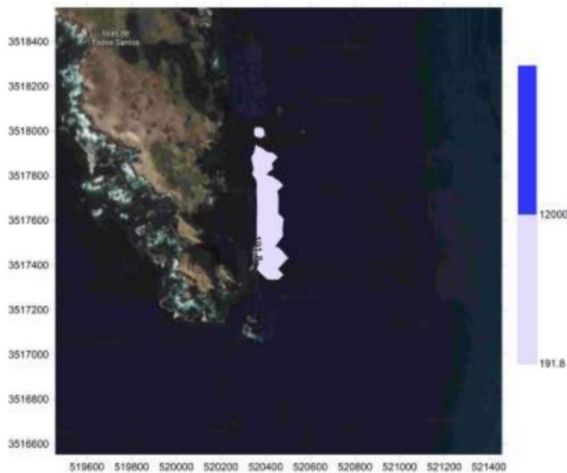
Figure 11: Modeling of area receiving > 191.8g/m 2 /year at a realistic stocking density of 20 kg/m 3 , therefore exceeding SEPA’s threshold of “change or degradation” of benthic communities. The blue threshold of 12,000 g/m 2 /year was not reached.
